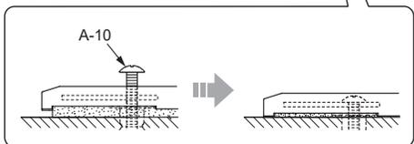
Failure to tighten screw A-10 completely will cause moving sideways of C-1.
