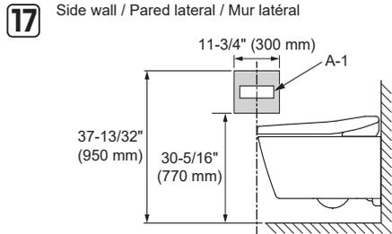
**18** Temporarily place the remote control in the position determined in **17** and confirm the signal reception of A-1.
